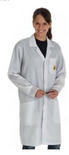
Long sleeves, 3/4 design with 2 side pockets, conductive 4 mm grid, polyester fabric (98% polyester, 2% carbonized yarn), breast pocket with woven ESD symbol, continuously covered snap fastener. Machine washable up to 40°C, weight 120 g/m<sup>3</sup>. Suitable for clean production areas.
