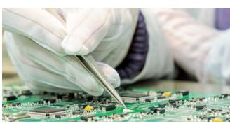
The gloves made of polyester with woven, conductive carbon fibers have good dissipation values and are suitable for the use in cleanrooms.
