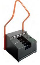
Four counter-rotating wheel brushes clean the soles from underneath. Two lateral disk brushes clean the edges of the soles. The brushed-off dirt falls into a large drawer at the bottom of the device. This drawer can be removed and cleaned
