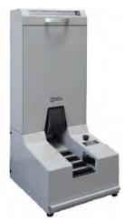
Four wheel brushes clean the soles, while the two lateral disk brushes clean the edges of the shoes. The uppers are cleaned by a third brush. The brushed-off dirt falls into a large drawer that can be cleaned easily. A round belt drive ensures a powerful brushing while running smoothly at the same time.
