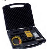
$\mathsf{EFM}^*\mathsf{51}$  with conductive base and measuring head MK 51. By attaching the measuring head MK 51 EFM can be used for the verification measurement of the body voltage (walking test)\* according to IEC 61340-4-5. The measuring head MK 51 is specially calibrated to the EFM°51. The positive and negative "PEAK" value of the measured body voltage is displayed
