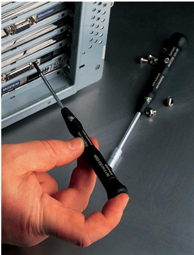
The handle sleeves do not provide any protection against voltage.
