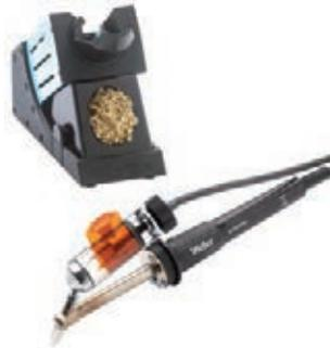
Due to its design the desoldering iron DSX 80 offers an ergonomic posture and a fatigue-free working even during longer use. The solder collector can be cleaned quickly and easily. The vacuum is activated by the finger switch integrated in the handle. A wide range of nozzles and CSF heads makes it a universal tool.
