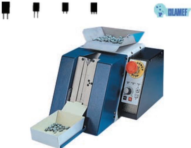
Loose radial components can be cut with the TC 4 cutting machine.
