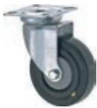
**Bracket:** heavy pressed sheet steel bracket, galvanized; fork head with double ball bearing; bolted axle; with top plate.
