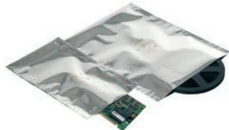
JEDEC protective bag, non-transparent, water-impermeable, aluminized moisture barrier bag, offers an excellent protection against moisture as well as static charge due to a special multilayer made of nylon, polyethylene and aluminium.
