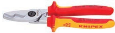
VDE-tested cable shears, hardened cutting edges with precision grinding, cuts smoothly and cleanly without squeezing. Minimum effort by favorable lever ratio, easy cutting by one-hand operation, trap protection, adjustable screw joint, self-locking.
