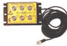
Grounding box with 6 ports, for use as central grounding reference point, grounding wire 2.5 m with screw eye M4, mounting plates, each port 1 MOhm safety resistance
