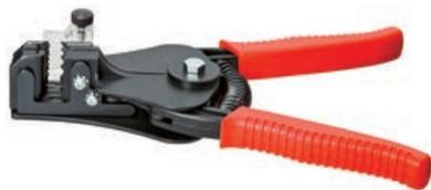
Gentle stripping of fine wires, clamping jaws hold the wire while stripping. Length stop for constant stripping lengths in serial work. Pressure spring to reach the starting position, robust light metal body.
