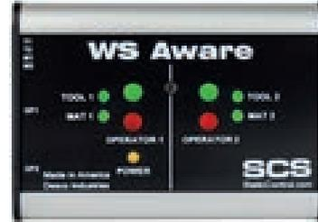
**WS Aware workstation monitor allows the permanent monitoring of two workstations.** The measuring device equipped with a DSP (digital signal processor) monitors the flawless ground connection of users, tools and working surfaces. Furthermore, EMI events are registered and displayed. WS Aware monitors detect all grounding parameters of the working environment in accordance with the requirements of ANSI 6.1 and ANSI/ESDA S. 20. 20.
