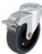
**Bracket:** sheet steel bracket with bolt hole 13 mm, double ball bearing in the swivel head, sturdy central bolt, axle bolted, galvanized/chromated, lock "stop-fix".
