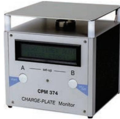
The Charged Plate Monitor CPM 374 measures the voltage potential on its integrated plate electrode. The monitor is suitable to determine the discharge time from a preset voltage threshold to a lower voltage value level. A timer, a high voltage unit and an electric field meter working according to the fieldmill influence principle are integrated. This allows for the necessary high input impedance of  $10^{15}\Omega$  to measure electrostatic voltage potentials and discharge times of air ionizers.
