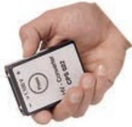
Handy instrument used to measure the effectiveness of ionizers and those offset voltage ⚠
