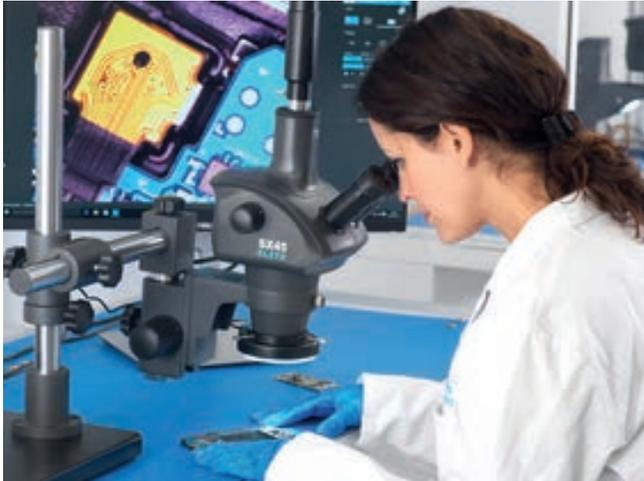
High-quality stereo zoom microscope with optical Greenough principle for a wide range of applications impresses by a solid, durable design and its easy operation. The image remains in the exact level of sharpness throughout entire zoom range.
