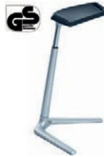
ESD standing aid Fin with solid foot, seat height adjustment by Safelift gas spring in the range of 620-850 mm, pillar for an ideal working position and ergonomic support tilted forwards by 4°, extra wide comfort seat (turnable by 20°) with integrated handles, integral foam upholstery black.
