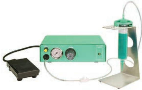
The analog dispenser DC150 is only recommended for manual dispensing applications. The dispensing process is triggered by pressing the foot switch. The device is a low-cost alternative and ensures continuous dispensing operations with the same precision and quality. It is suitable for all types of media and equipped with vacuum retention to that to avoid dripping of low-viscosity media.
