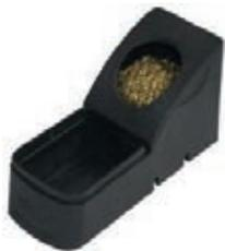
The solution for cleaning problems with lead-free solders by special metal wool. Primary cleaning of the soldering tip by tapping it in the collecting tray, fine cleaning by brushing and turning in the spiral wool.
