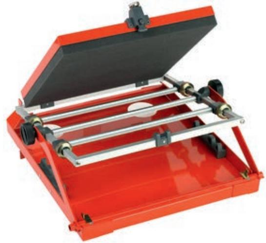
The assembly frames facilitate the equipping and soldering of PCBs, especially for series production.
