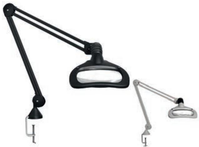
The Wave LED is an illuminated magnifier for industrial applications, with 2 x 6 Watt LED light sources and a flexible self-balancing arm. It offers shadow-free magnification with light coming from both sides, as well as three-dimensional magnification with light coming from the left or right.
