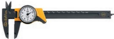
Scale 0.1 mm, made of electrostatically dissipative material, shock-proof dial, round scale adjustable to zero, comparative measurements possible. Outdoor, indoor, depth and stage measurements, for all working on electrostatically sensitive components.
