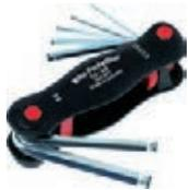
7-piece fold-out holder, galvanically finished blades with MagicRing®, made of spring steel (from size 3 mm); holds all standard screws in each position, ballpoint allows the screwing at an angle of up to 25°.
