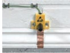
Grounding connection set for floor coverings for wall mounting with test point (socket 4 mm) and 2 m self-adhesive copper tape, for the grounding of an area up to 10 x 20 m. Grounding wire 3 m with eye.
