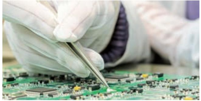
The gloves made of polyester with woven, conductive carbon fibers have good dissipation values and are suitable for the use in cleanrooms.
