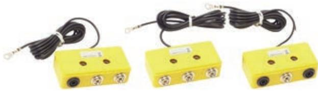
Grounding box with 3 laterally mounted ports, for use as central grounding terminal, grounding wire 2 m with screw eye M4, each plug 1 MOhm safety resistance
