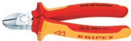
VDE-tested versatile diagonal cutting pliers, slim head shape with precision cutting edges for a clean cut on soft and hard wire. Precisely processed, made of high-quality vanadium electric steel.
