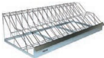
The reel rack is suitable for SMD reels with 180 mm, 330 mm and 380 mm Ø. SMD reels with 180 mm Ø can be arranged in two rows (max. 60 reels per row). The rack has 15 compartments that are 60 mm wide. The steel wire dividers have a conductive powder coating. Load capacity 50 kg.
