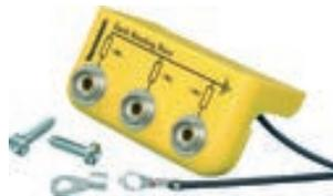
Grounding box with 3 ports, laterally mounted at right angle, as central grounding terminal, grounding cable 3 m with screw eye M4 / plug 1 MOhm safety resistance per port LxWxH: 72x37x38mm
