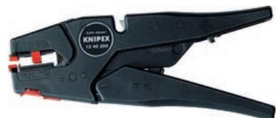
For single, multi- and fine-wired conductors insulated with plastic/rubber. Automatically adjusting to conductor cross-section. Cutting depth readjustable. Smooth-running mechanism, easily exchangeable blades and plastic clamping jaws with wire cutters (multi-wired up to 10 mm<sup>2</sup>, single-wired up to 6 mm<sup>2</sup>), low weight, case made of tough, glass fiber reinforced plastic.
