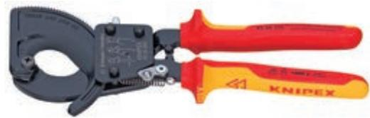
VDE-tested cable shears, hardened cutting edges with precision grinding, cuts smoothly and cleanly without squeezing. Two-stage ratchet drive for easy cutting. Minimum effort by favorable lever ratio, trap protection, adjustable screw joint, self-locking.
