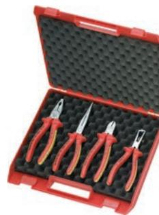
4-piece, contains 4 VDE-tested pliers. High-quality and versatile, impact-resistant plastic suitcase, napped foam insert for variable equipment. (Dimensions WxDxH: 327x275x65 mm)
