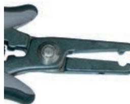
Special pliers, developed for the forming of the components in a C shape. Its special radius allows a stress-free forming of components. Length 150mm. Max CU Ø 1.02 mm, 18 AWG
