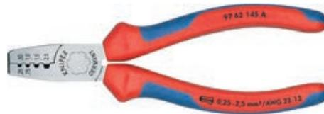
Wire end ferrule pliers for the crimping of wire end ferrules according to DIN 46228 parts 1 + 4, crimping in marked trapeze profiles for a safe connection of sleeve and conductor, vanadium steel.
