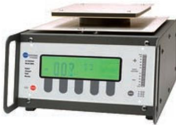
Charged Plate Monitor 280A is used to measure the effectiveness of ionizers and their offset voltage
