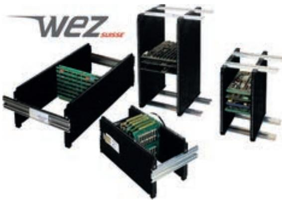
Simple and safe system for PCB handling in the production, in the storage and for the transport. Modular design fits in Euro containers. Individually configurable for the different practical needs.
