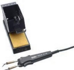
The desoldering tweezers WTA 50 were designed to desolder SMD components and can be connected to all Temtronic stations. Two heating elements with their own temperature sensor ensure uniform temperatures on the two legs. The tips are fixed by clamping screws.
