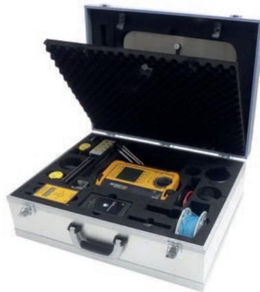
Audit set for the measurement and control of protective components in ESD protected areas.
