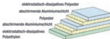
Water-impermeable, metallized barrier bag, offers an excellent protection against moisture and static charge by a special multilayer of dissipative polyethylene and polyester as well as metallized polyester film
