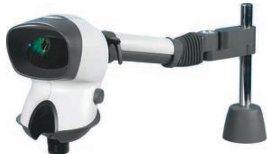
For general incident light applications with magnification x2 to x20 (option), inspection and rework "freehand" on small and large parts from all technical fields, great flexibility by specially designed articulated arm, single-station system with clamping or 3-hole mounting on the workstation. For magnifications of x10 and higher the use of the table stand MBS-002 is recommended.
