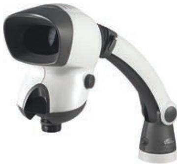
For general incident light applications with magnification x2 to x20 (option), inspection and rework "freehand" on small and large parts from all technical fields, single-station system with clamping or 3-hole mounting on the workstation. For magnifications of x10 and higher the use of the table stand MBS-002 is recommended.
