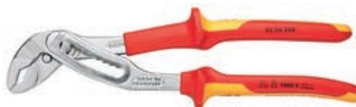
Insulated, VDE tested, high stability, self-clamping on tubes and nuts; trap protection prevents contusions, favorable leverage for optimal power transmission; gripping surfaces with specially hardened teeth (61 HRC), chrome-vanadium electric steel.
