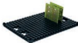
PCBs of every size are safely held in the plug-in / knobbed board, electrostatically conductive volume, knobs: round Ø 16 x 6 mm, max. PCB thickness 1.6 mm
