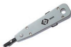
For the insertion of telecommunication and data cables into terminal clamps; wires are crimped and cut in one single operation; suitable for a variety of different terminal blocks e.g. crowns and similar products; handle contains a wire extractor hook and a grooving tool
