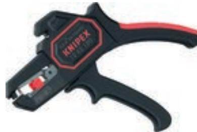
Compact standard tool with slim head shape; for single-, multi- and fine-wired conductors; automatic adjustment to the conductor cross-section; high ease of use due to the handy and light design; length stop, wire cutters up to 2.5 mm<sup>2</sup>, easily exchangeable blades, case made of tough, glass fiber reinforced plastic; with ergonomic soft plastic zone in the handles.
