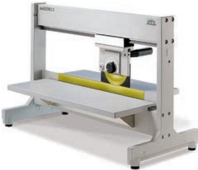
The MAESTRO 3E separates large and small PCBs. The table and the rest are steplessly adjustable to the best working position. The distance between linear blade and the rest can be adjusted in such a way that the edge strips fall through and sorted out.
