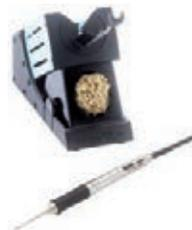
The Weller soldering pencil WMPR achieves its operating temperature in a very short time. Exchanging the soldering tip is possible without tools. When the iron is placed in the WMRH safety rest, the temperature is immediately switched off, which increases the service life significantly. Suitable for soldering stations WMRS, WD 1 M, WD 2M and WR 3M.
