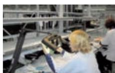
With the magnifier lamp SNLQ 54/2 A it is possible to modify basically the lighting character by switching the LED. This allows to execute all inspections with only one lamp.
