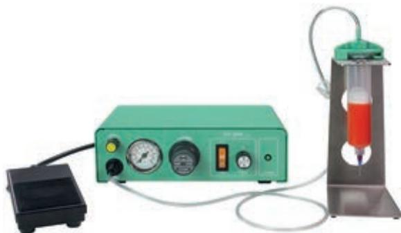
The devices of the **DC 200 dispenser series** are equipped with a timer allowing to adjust a dosing time of 0.01 to 30 seconds. The two available versions can be distinguished by the dimensioning of the compressed air outlet. The DC 200 is designed to control precisely the pneumatically controlled dosing cycles, like e.g. dosing cycles of 3 – 55 cc small cartridges. The integrated pressure regulator allows for a precise pressure.
