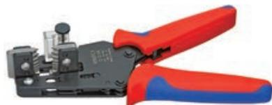
Easy stripping of difficult-to-process insulating materials such as Teflon®, silicone, RADOX®, Kapton® and rubber as well as multi-layer insulation. No damaging of conductors by precisely ground forming blades. Gentle stripping of fine wires; length stop, smooth-running mechanism, high ease of use due to the handy, compact design; 4 exchangeable blades.
