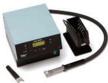
Built-in turbine, so independent of compressed air. Digital control electronics, LCD display, manual or automatic operation, RS 232 interface for control via PC, connection for external sensor, max. nozzle vacuum -0.6 bar, safety rest with Stop + Go function, protection class 1.
