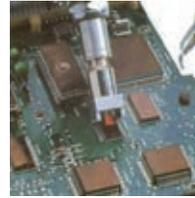
The vacuum is activated by a finger switch and the solder is collected in integrated collecting box. When using SMD desoldering heads, the component is lifted with the integrated vacuum. The hot air iron (HAP) is used for soldering with paste or for desoldering. In this case, smaller components can be evenly heated with the standard nozzle; however, larger devices can be desoldered with a suitable nozzle.
