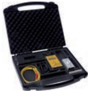
EFM®51 with conductive base and measuring head MK 51. By attaching the measuring head MK 51 EFM can be used for the verification measurement of the body voltage (walking test)® according to IEC 61340-4-5. The measuring head MK 51 is specially calibrated to the EFM®51. The positive and negative "PEAK" value of the measured body voltage is displayed
