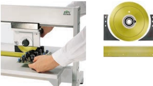
The pre-scored groove can arbitrarily be interrupted by cut-outs.
