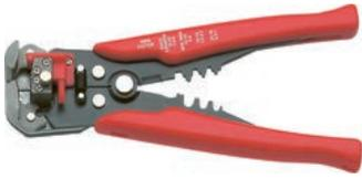
for the stripping, cutting and crimping of wires; hardened steel blades for a long service life; automatic stripping of wires without adjustment; crimping of insulated and uninsulated terminal clamp; micro adjusting knob allows the stripping of wires of less 0.2 mm<sup>2</sup>.
