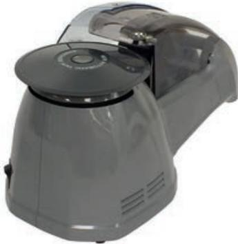
Universal tape dispenser type A619 with electrical drive and rotary table, for adhesive tapes from 3 to 25 mm range. Cuts length from 10 to 61 mm. Suitable for each roll length until max. 150 mm Ø.
