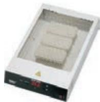
Digital display of nominal and actual temperature, digital control electronics, 3 infrared high-temperature radiator for a fast and efficient heating, 2 heating zones selectable, external sensor (accessory) connectable, RS 232 interface for the connection to WHA 3000 hot air station (control over WHA 3000P), temperature range 50° - 400°C, heated surface 120 x 190 mm or 190 x 245 mm, ESD safe.
