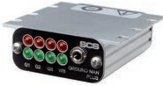
The **Ground Man Plus** monitors can be used to control the grounding impedance of workstations, tools and machines. The grounding impedance of up to 3 connectors against hard grounding can be monitored.
