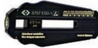
Adjustable ESD Precision stripping tool, made of dissipative material; adjustable to each 6 cable diameter; suitable for PVC, Teflon and other material; 50 mm scale with 1 mm division and adjustable length stop; specially hardened blades
