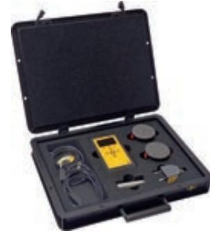
Verification kit for the measurement of conductive/dissipative surfaces
