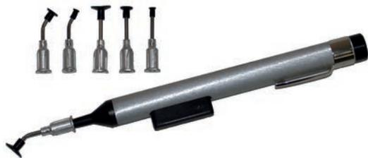
With this PEN-VAC, a vacuum pipette without external pump, it is possible to lift, to transport and putting down small components with a smooth surface up to a weight of 200 g. The pipette itself has a weight of less than 50 g. It is smaller than a ballpoint pen and is equipped with a clip. A reserve sleeve for suction nozzles and rubber is available.
