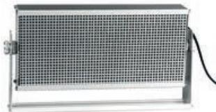
Due to its oblong design and the high air flow rate, this device is optimal for manual soldering stations in the PCB production. The extractor is delivered complete with a mounting bracket.
