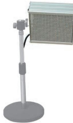
This solder fume extractor was designed to absorb harmful fumes at the workstation. It prevents actively headaches, inflammation of the eyes and fatigue often caused by the inhalation of solder fumes. The powerful axial fan extracts the malodorous solder fumes through a activated carbon filter. Chemical pollutants are absorbed effectively.
