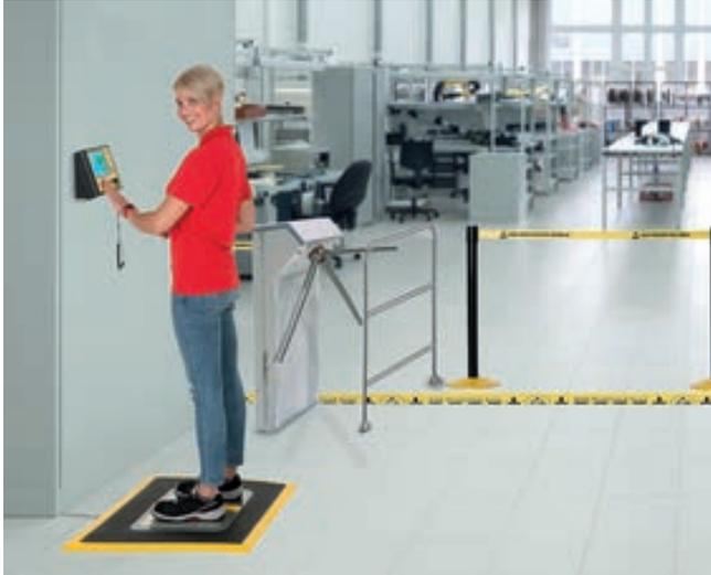
In combination with the modern EPApro® personal grounding test system it is possible check and document the function of the personal ESD protective equipment when accessing an EPA protected zone.
