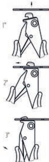
This handy off-cut remover tool allows the quick separation of milled PCBs.
