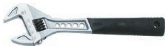
with "Sure Drive" mouth profile - grips the screws heads and nuts at the sides and not at the corners thus avoiding a "spinning"; made of chrome-vanadium steel, matt chromed - especially robust and protected against rust; comfortable soft handle; metric and inch scale / mouth 18% wider than the standard models. With advices concerning the direction of rotation to protect the screws.
