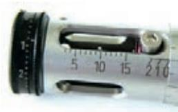
The high-precision stripping tool MiniStrip is quickly adjusted to different diameters and lengths by a calibrated scale. A locking screw allows the blocking of the diameter adjustment. The high-quality processing guarantees an accurate repeatability of the tool.
