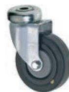
**Bracket:** heavy pressed sheet steel bracket, galvanized; fork head with double ball bearing; with bolt hole
