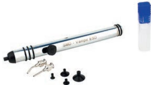
The pick-up tool "VAMPIRE" is a handy and battery-free tool, ideal for the handling and positioning of SMD components. Excellent suction capacity and its high-performance suction nozzles allow the lifting of components up to the weight of 120 g. Due to the electrical conductivity of all components, the pick-up tool "VAMPIRE" can be used in ESD protected areas.
