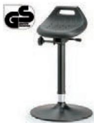
ESD standing aid with solid flat round base, seat height adjustment by Safelift gas spring in the range of 650-850 mm, tilt adjustment forwards by 10°, 360° rotatable lean-to surface made of conductive integral foam with integrated handle. Metal parts coated with epoxy resin, color: black.
