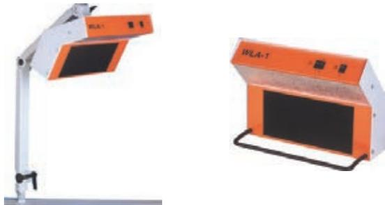
The WLA 1 LED soldering fume extractor absorbs the harmful fumes, gases and vapors produced during the soldering process, and cleans the polluted air immediately at the workstation with a Poret®-Carbon activated carbon filter.
