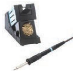
The WP 80 soldering iron convinces by its short shape, which is a big advantage for soldering work under the microscope. The distance from the handle to the soldering tip shaft is only 40 mm.
