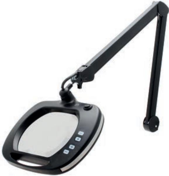
The LE-WUVE5D lamp has unique illumination options allowing the user to use UV LEDs or standard white. The UV LED lamps work with 400 nm and can be used to inspect protective paint, holograms etc. (for every type of material fluorescing during inspection). This model has more than 48 adjustable white LEDs as well as 30 UV LEDs. It is equipped with an ESD-safe coating providing dissipation of static energy to protect sensitive components.
