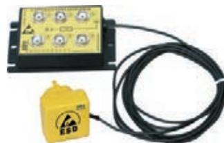
Grounding box with 6 ports mounted at the top, as a central grounding reference point, mounting plates, grounding wire 2.5 m / plug with plastic holding pins
