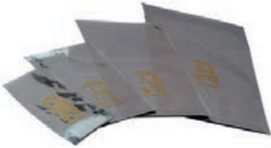
Metallized, transparent shielding bag, aluminized, interior PERMASTAT®, permanently antistatic and amine-free polyethylene, side welded seam, heat-sealable, recyclable, standard imprint: ESD symbol, type designation, recycling symbol and lot number.
