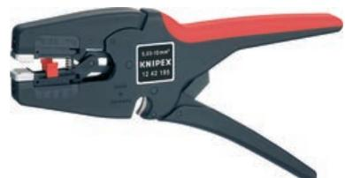
Fully automatic adjustment to the different insulation thicknesses depending on the cross-section; automatic setting of the cutting depth; clamping jaws made of steel with integrated cutting edges, with wire cutters (multi-wired up to 10 mm<sup>2</sup>, single-wired up to 6 mm<sup>2</sup>); tough, glass fiber reinforced plastic case.
