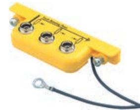
Grounding box with 3 ports, laterally mounted, flat design (depth 17 mm) as a central grounding terminal, grounding wire 2 m with screw eye M4 / plug 1 MOhm safety resistance per port LxWxH: 110x38x17mm
