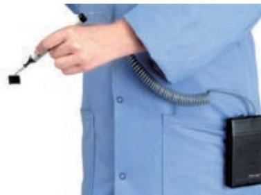
Portable vacuum handling system, battery-operated (9V alkaline, 8 hours operating time), with 1.2 m spiral hose wire ( $\varnothing$  1.6 mm), set with 7 vacuum tips VCS-7-B, vacuum pipette V3020-RF-1/16, with belt / pocket clip on the housing, weight 156 g.
