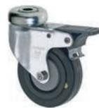
**Bracket:** heavy pressed sheet steel bracket, galvanized; fork head with double ball bearing; with double stop; with bolt hole
