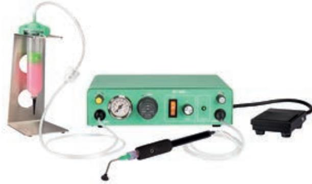
The vacuum tweezers turn the **DC 600** into the ideal device for pick-and-place applications and for the mounting and reworking of small components. Before positioning the components it is possible to apply solder pastes and other materials with maximum precision. so, the DC600 is suitable for many industrial applications in the miniature field. It is suitable for all types of media. The device is equipped with a vacuum retention system to avoid a dripping of low-viscose media.
