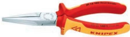
VDE-tested long-nosed pliers, highly-resistant and low-wear. Long, flat jaws with serrated gripping surfaces, made of chrome-vanadium electric steel.
