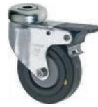
**Bracket:** light pressed sheet steel bracket, galvanized; fork head with double ball bearing; with double stop; with bolt hole
