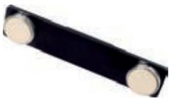
for surface resistance measurement of vertical surfaces with a specified distance of 30 cm; connectable to a high-speed ohmmeter; conductive contact rubber with silver particles; weight: 950 g; dimensions: 385 x 85 x 70 mm (LxWxH); contact rubber:  $\varnothing 63.5$  mm
