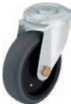
**Bracket:** sheet steel bracket with bolt hole 13 mm, double ball bearing in the swivel head, sturdy central bolt, axle bolted, galvanized/chromated.
