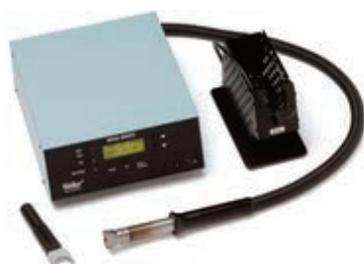
Requires 4-6 bar compressed air or protective gas supply. Digital control electronics, LCD display, manual or automatic operation, RS 232 interface for control via PC, connection for external sensor, max. nozzle vacuum - 0.6 bar, safety rest with Stop + Go function, protection class 1.
