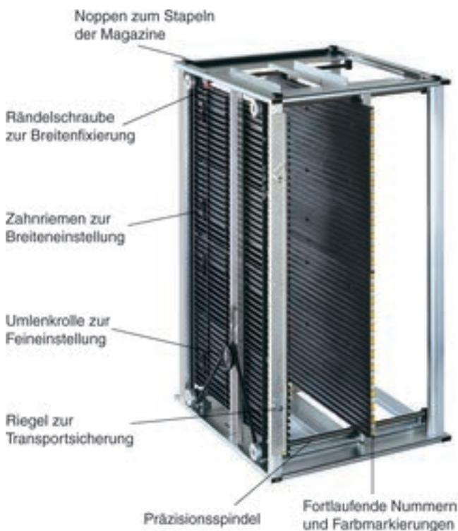
Version conductive = electrostatically volume conductive
