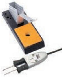
The WMRT desoldering tweezers allow a precise soldering and desoldering of very small SMD components by its pairwise, parallel adjusted soldering tips. When placed in the safety rest WMRTH with Stop+Go function, adjustable soldering tips are switched off, which increases the durability.
