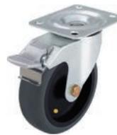
**Bracket:** sheet steel bracket with top plate, double ball bearing in the swivel head, swivel head sealing, axle bolted, galvanized/chromated, lock "stop-fix".
