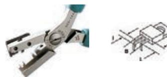
Bends components T0126, 218, 220 power transistors, etc. by 90° on two rows. Adjustable with screw.
