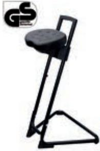
Sit-stand stool; dissipative, stable support tube with slip-resistant glides; lockable seat height adjustment; seat tilt adjustable by 15°; dissipative, durable seat made of PU integral foam; rotary movement of the seat by 16° ensures good contact; GS approved. Color black.
