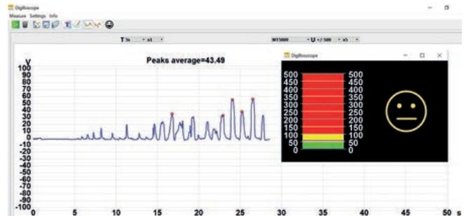
The walking test kit is used mainly to measure the body voltage and their graphical presentation.
