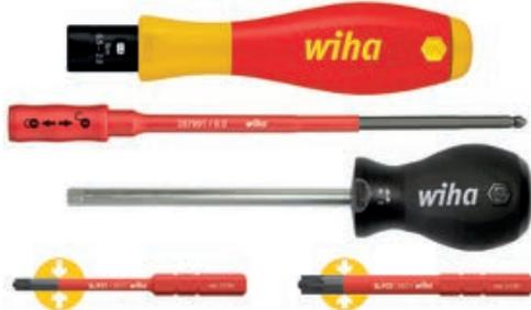
5-pcs torque screwdriver set Torque. Controlled fastening on live parts up to 1,000 V AC. VDE torque handle steplessly adjustable with Torque Setter adjusting tool (included in the scope of delivery) from 1.0 - 5.0 Nm. Protective insulation molded directly onto the bit and completely integrated into the bit in the lower area.
