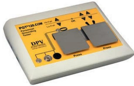
The personnel test station PGT®120.COM tests personnel bleeder resistances for the access control to your ESD-protected area. PGT®120.COM has an additional RS232 interface for the connection to a PC or a terminal. The data is transmitted in ASCII format. A PC with terminal program is sufficient to display the measured data.
