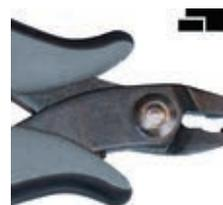
Special pliers for the electronics. In only a single operation, the component is cut, bent and at the same time blocked on the printed circuit board.
