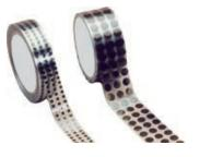
High-temperature resistant polyimide foil, silicone adhesive Thickness incl. adhesive approx. 0.070 mm Thermal class H 180°C, heat resistance 240°C/10 min, temporarily max. 260°C Color: brown transparent
