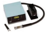
Requires 4-6 bar compressed air or protective gas supply. Digital control electronics, LCD display, manual or automatic operation, RS 232 interface for control via PC, connection for external sensor, max. nozzle vacuum - 0.6 bar, safety rest with Stop + Go function, protection class 1.
