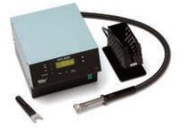
Built-in turbine, so independent of compressed air. Digital control electronics, LCD display, manual or automatic operation, RS 232 interface for control via PC, connection for external sensor, max. nozzle vacuum -0.6 bar, safety rest with Stop + Go function, protection class 1.
